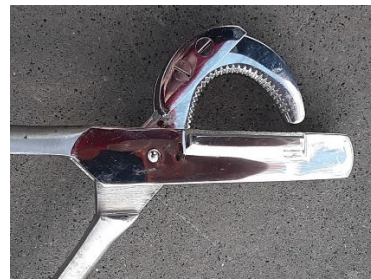
Figure 2: This photo illustrates the crushing grooves found on the back surface of the blade. Photo taken by Sandy Stuttgart Extension Taylor County.
