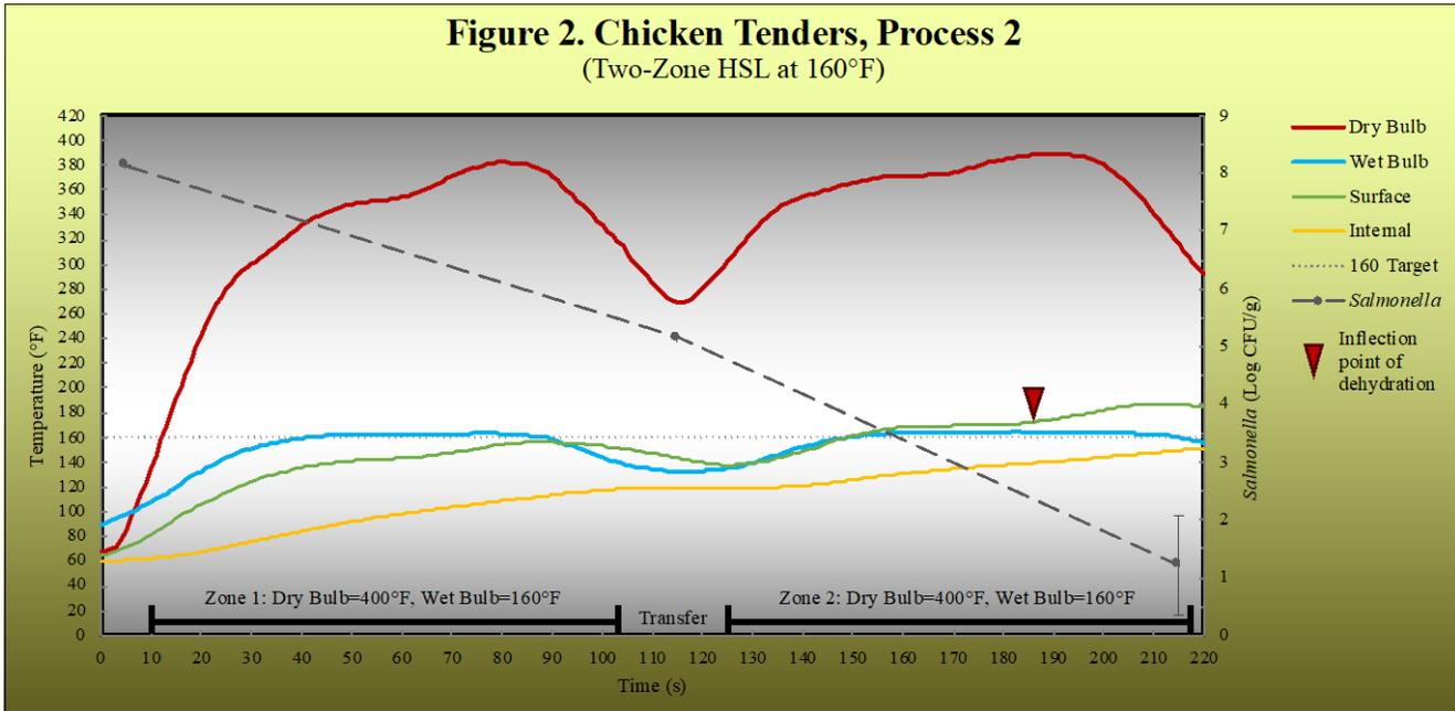
bulb temperature. Processes 2 and 7 used the shortest cooking time of 3.0 minutes, compared to 3.5 minutes for Processes 3-6 and 4.0 minutes for Process 1, but still exceeded the targeted  $\geq 6.5$  log reduction of *Salmonella* for all products investigated.
