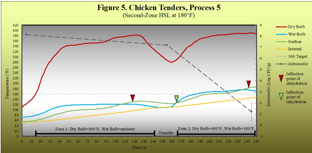
tenders exceeded the wet-bulb temperature near the end of Zone 1, indicating that the surface was beginning to dry and had transitioned into the falling-rate drying period by the end of the zone.
