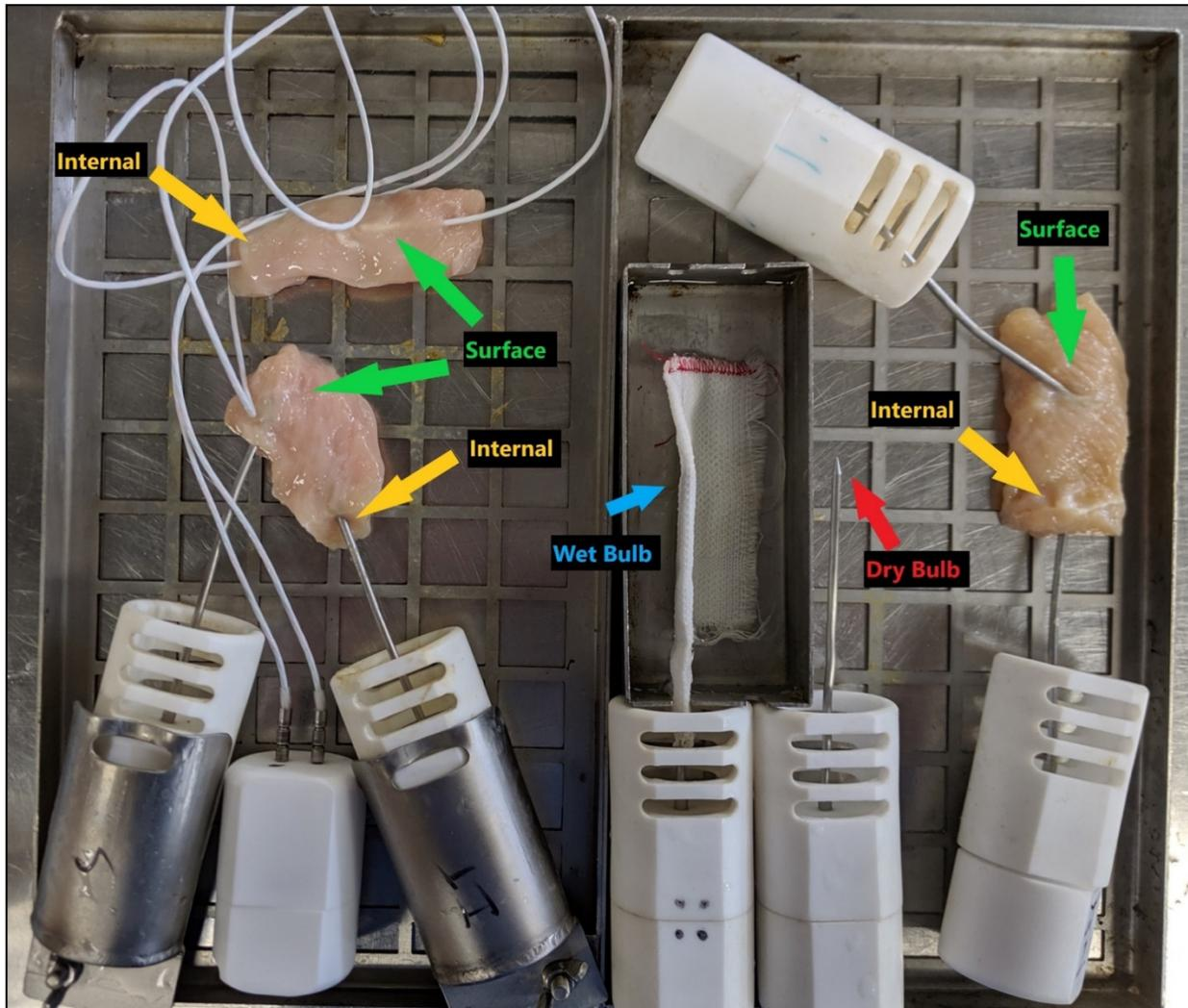
**Diagram 2.** Data logger placement for measurement of product surface and internal temperatures.
